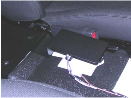
Position sensor guard to align with OEM floor nutserts (Item 5)
